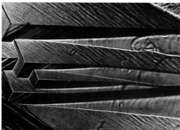
Fig. 4. The fish-shaped structure produced by etching ( \times 200 ).
