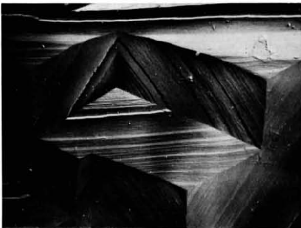
Fig. 3. Joining of opposite wings of two etch pits ( \times 4800 ).
