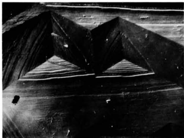
Fig. 2. An etch pit with two wings ( \times 4800 ).
